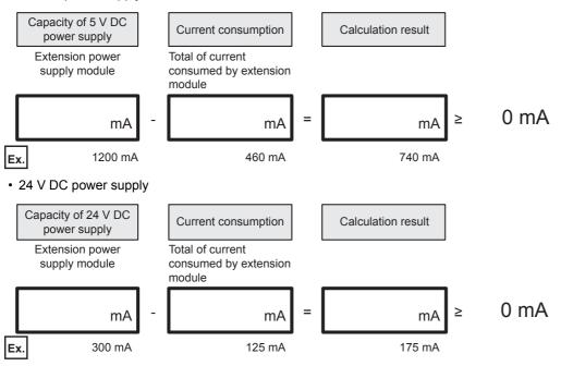
If the calculation result is a negative value, the current consumption exceeds the power supply capacity of the extension power supply module.
