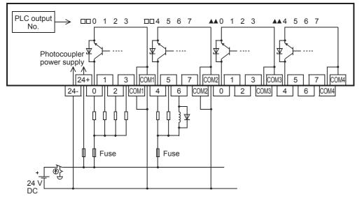
For external wiring precautions, refer to F Page 123 Wiring precautions.
