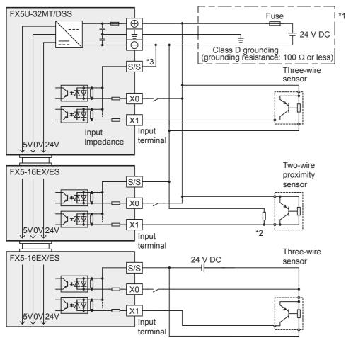
\*1 Handle the power supply circuit properly in accordance with "Power Supply Wiring."
