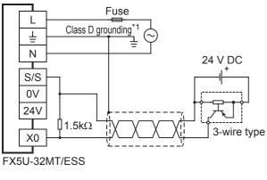
\*1 The grounding resistance should be 100  $\Omega$  or less.
