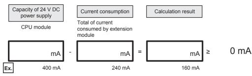
If the calculation result is a negative value, the current consumption exceeds the power supply capacity of the CPU module. Reconfigure the system, adding powered input/output module or extension power supply modules.
