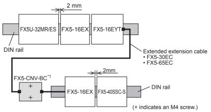
\*1 FX5-CNV-BC can only be installed directly.
