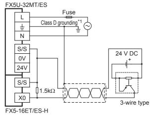
In the case of source wiring
