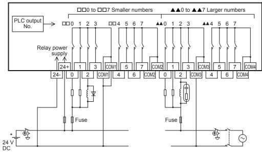
For external wiring precautions, refer to F Page 126 Wiring precautions.
