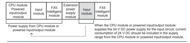
3. Calculate the total current consumption of each power supply.
