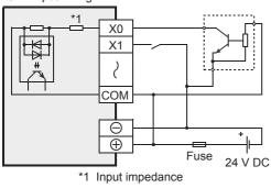
In the source input, the input (X) is turned on by connecting 24 V DC [-] with the [COM] terminal, and connecting a no-voltage contact or PNP open collector transistor output between the input terminal and 24 V DC to close the circuit.
