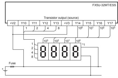
\*1 Use a 7-segment display with a latch and a built-in BCD decoder.
