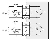
Source output Connect +V□ (number) terminal to the plus side of the load power supply.
