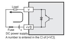
For the output module (extension connector type) and input/output module (extension connector type), the transistor output
