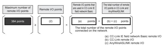
The maximum number of remote I/O points differs according to type of the network.
