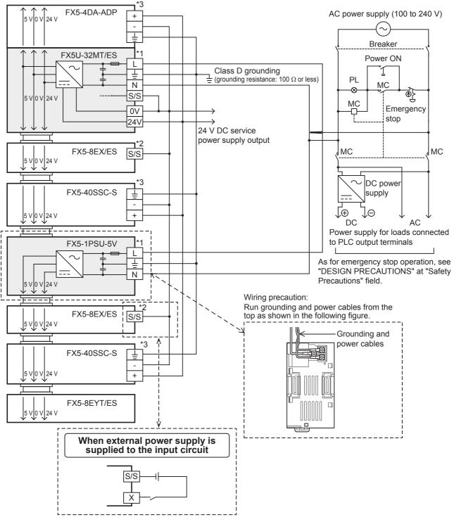
\*1 Connect the AC power supply to the [L] and [N] terminals (common for 100 V AC system and 200 V AC system). Make sure that the power of the FX5-1PSU-5V is turned on at the same time as the CPU module or earlier than the CPU module.
