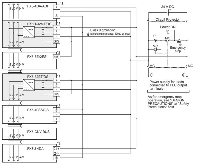
\*1 Connect the DC power supply to the [+] and [-] terminals. Make sure that the power of the powered input/output module is turned on at the same time as the CPU module or earlier than the CPU module.
