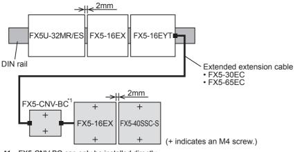
\*1 FX5-CNV-BC can only be installed directly.
