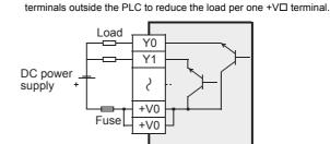
The +VD (number) terminals that are connected each other inside the
