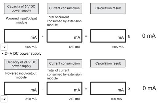
If the calculation result is a negative value, the current consumption exceeds the power supply capacity of the CPU module. Reconfigure the system, adding powered input/output module.
