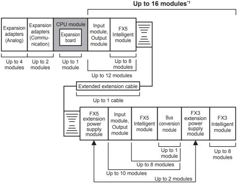
\*1 Extension power supply modules and connector conversion module are not included in the number of connected devices.
