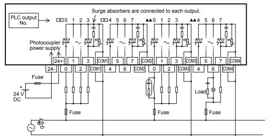
For external wiring precautions, refer to F Page 126 Wiring precautions.
