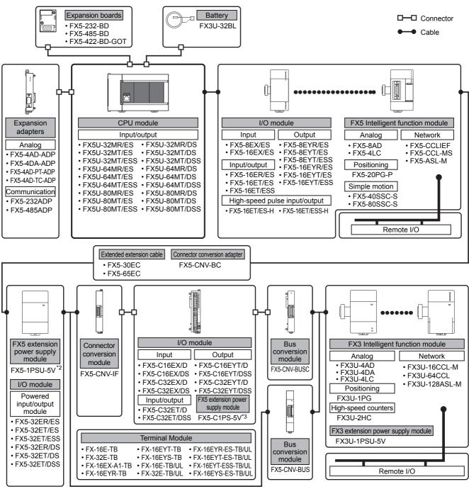
\*1 Use this to connect a module (extension cable type) located distantly or on a second stage. The connector conversion adapter (FX5-CNV-BC) is required when the connection destination is a module of extension cable type (except for FX5-1PSU-5V and extension power supply module). When also using a bus conversion module in the same system, connect the FX5-1PSU-5V or powered input/ output module directly after the extended extension cable.
