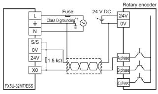
\*1 The grounding resistance should be 100  $\Omega$  or less.
