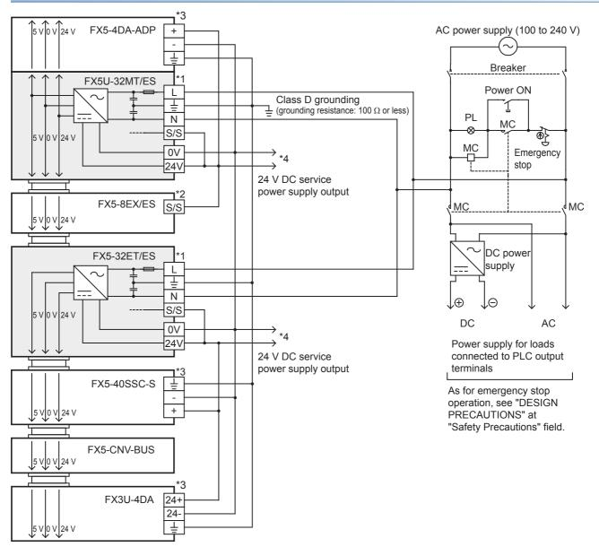
\*1 Connect the AC power supply to the [L] and [N] terminals (common for 100 V AC system and 200 V AC system).
