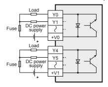
Source output [+common] Output to make load current flow out of the output (Y) terminal is called source output.
