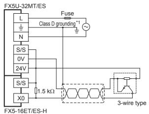
In the case of source wiring
