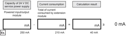
If the calculation result is a negative value, the current consumption exceeds the power supply capacity of the CPU module. Reconfigure the system, adding powered input/output module.
