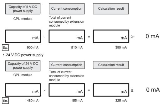
If the calculation result is a negative value, the current consumption exceeds the power supply capacity of the CPU module. Reconfigure the system, adding powered input/output module or extension power supply module.
