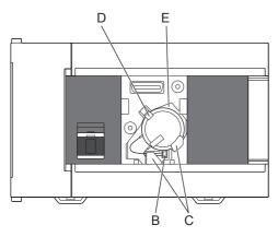
5. Attach the expansion board connector cover. If an expansion board was removed in step 2, reinstall it.
